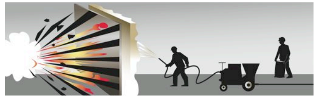
Figure1: Full scale blast testing simulation of Aquacrete VCD showing blast pressure
